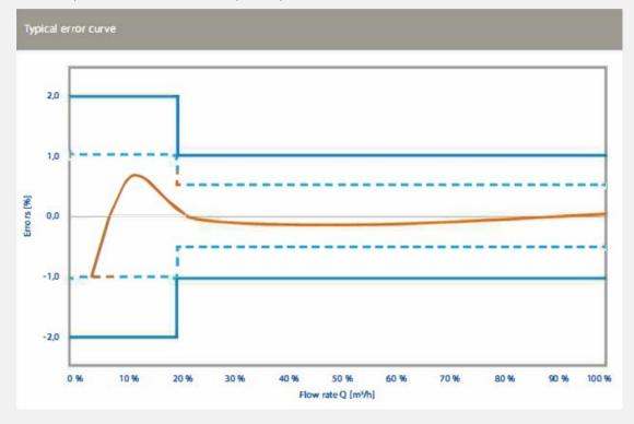
The turbine meters TBQM show very stable and reproducible measurement results.
